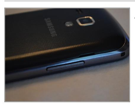
Locate the small hole on the left side of the phone near the volume rocker, which you can slip your fingernail into to pull the battery casing off.
