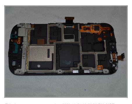
Voila! You now have exposed the belly of the beast! Or at least, the Thin Film Transistor housing.
