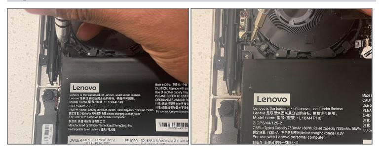
• Use the Phillips #0 screwdriver to remove the four screws securing the battery to the device.
