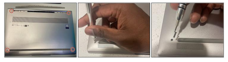
• Using the T5 Torx screwdriver, remove the four remaining screws on the outside of the frame.
