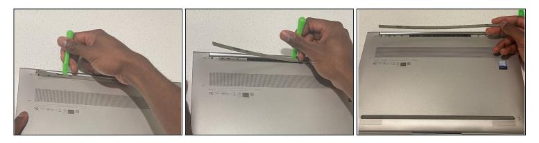
Using a plastic opening tool, remove the rubber foot.
