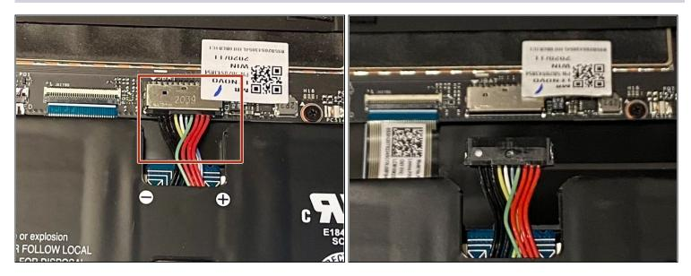
• To complete the removal of the battery, disconnect the ribbon cable connecting the battery to the computer.
