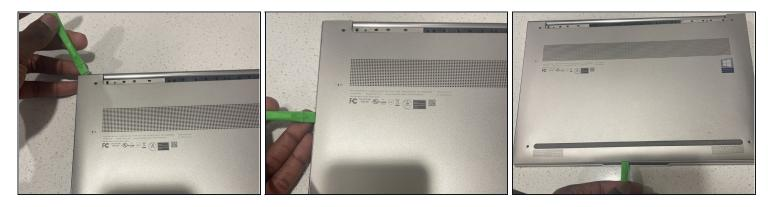
Starting at the top and working around, carefully pry open the bottom cover.
