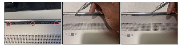
• Using the Phillips #0 screwdriver, remove the three screws underneath the rubber foot.
