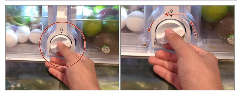
Rotate the knob of the filter counter-clockwise until the arrow lines up with the unlocked symbol.
