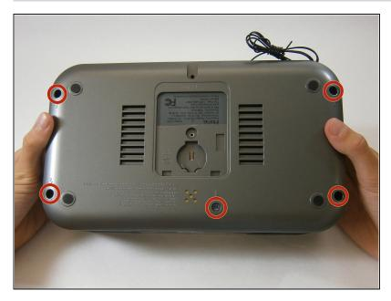
Unscrew five 17 mm-length, 6 mm-head screws using a Phillips #1 screwdriver.
