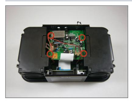
• Take out four 14 mm screws using a Phillips #1 screwdriver.
