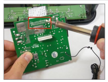
Desolder these 32 joints to detach the HDD data cable from the logic board.
