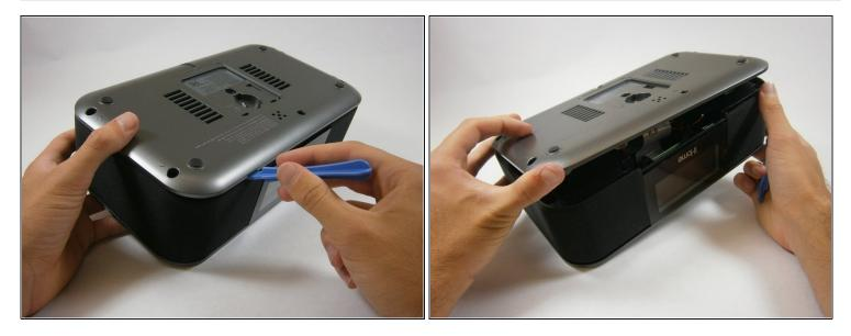
A The bottom cover is attached to the back cover by two plastic clips. Don't use excessive force.
