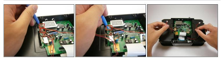
• Use a plastic opening tool to lift the two speaker zip connectors from the logic board.
