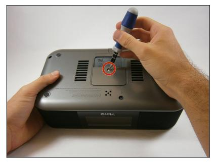
Remove the 10 mm-length, 5 mm-head screw using a Phillips #1 screwdriver.
