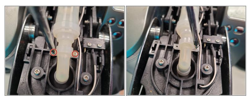
Using the Phillips #0 screwdriver, remove the two screws holding the tubing to the puncture needle.
