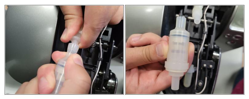
• Twist and pull to disconnect valve on the other side.
