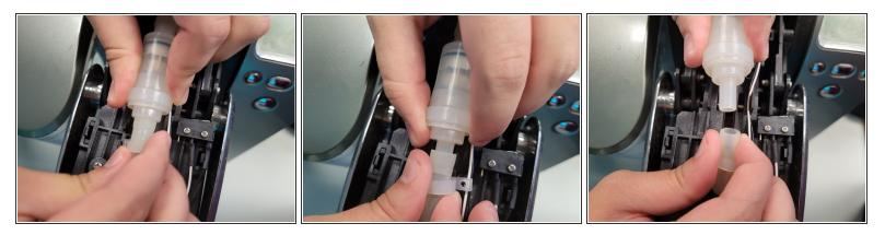
• Twist and pull to disconnect the valve on that side.
