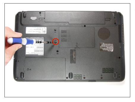
Turn laptop over and remove the 2.5mm "F3" screw using a Phillips #1 screwdriver.
