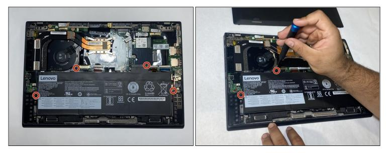
• Use the Phillips #1 screwdriver to remove the four 1.2 mm screws that secure the battery.
