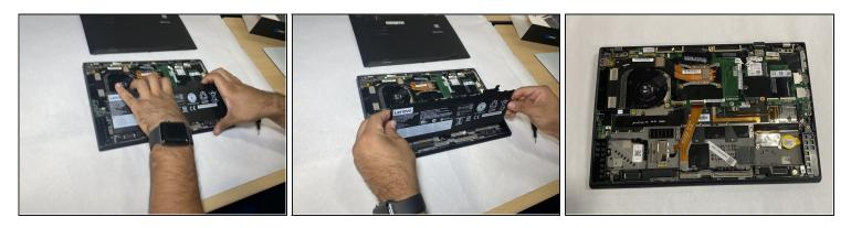
• Remove the battery using your hand or a prying tool.
