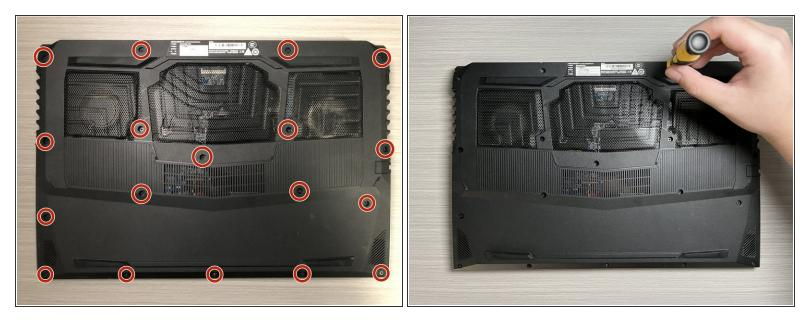
Using a Phillips screwdriver, remove eighteen 1.2mm Phillips #1 screws on the back.
