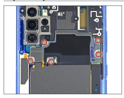
Use a Phillips screwdriver to remove the five 4 mm screws securing the wireless charging coil.
