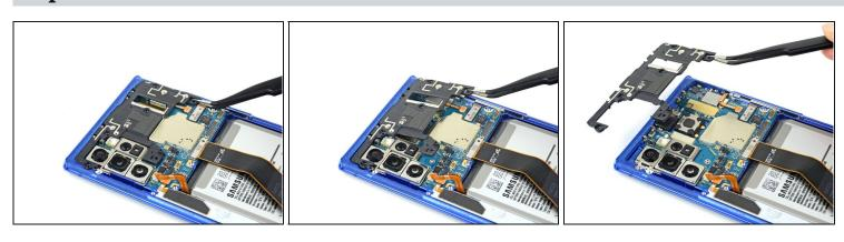
• Use a pair of <u>tweezers</u> to pivot the top plastic cover up and off of the phone.
