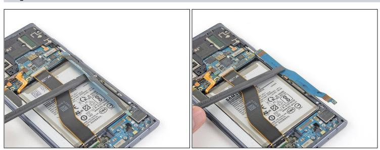
⚠ Don't try to remove the secondary interconnect cable. The cable is connected to the side 5G mmWave antenna.
