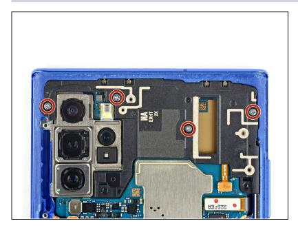
Use a Phillips screwdriver to remove the four 4 mm screws securing the top plastic cover.
