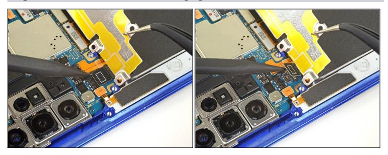
• Use the pointed end of a spudger to disconnect the wireless charging coil connector from the motherboard.
