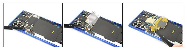
• Use a pair of <u>tweezers</u> to lift up and flip back the metal shield covering the battery connector.
