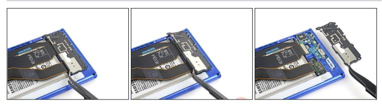
• Use a pair of <u>tweezers</u> to remove the loudspeaker.
