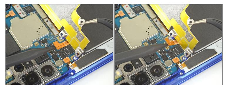
• While holding the metal shield up and out of the way, use the pointed end of a spudger to pry up the battery connector to disconnect it.
