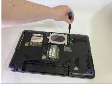
• Remove the four 6mm Phillips #00 screws scattered around the hard drive.
