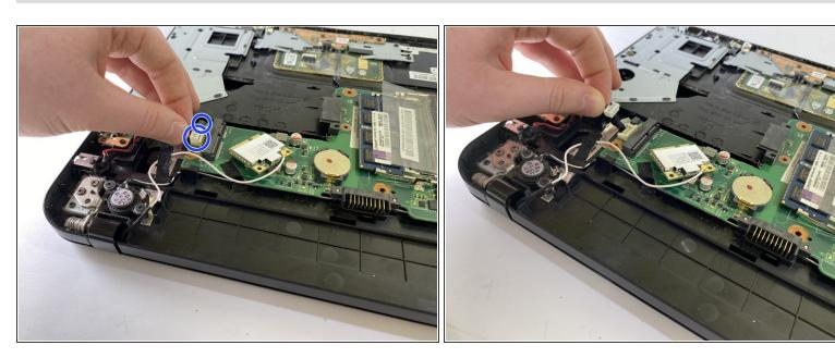
Disconnect the two cables for the DC power socket jack and the side usb board ribbon.
