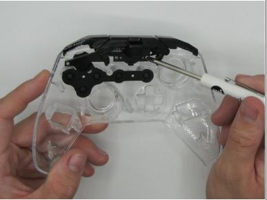
Remove the two screws from the top bumper board using a Phillips #1 screwdriver.
