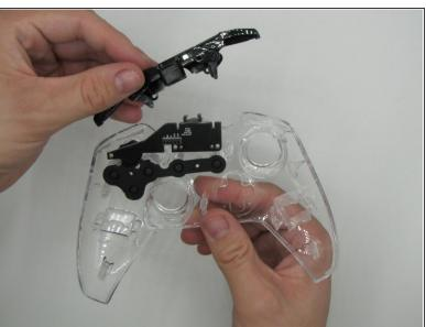
Pull up on the bumper board to remove it.
