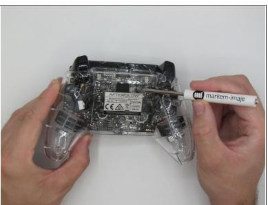
Remove the seven screws from the back of the controller using a Phillips #1 screwdriver.
