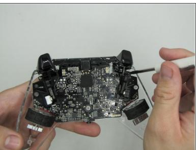
Remove both screws on the back of the motherboard under the triggers using a Phillips #1 screwdriver.
