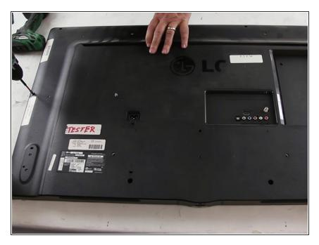
Reinstall the back cover and put the screws back in place. Removing and Reinstalling 4G LG TV LED Strips may sound tricky or complicated; however, after reading this tutorial for replacing the LED strips of LG 42inch LED TV, you can do it by yourself now! I hope you enjoy it. See you in the next tutorial.
