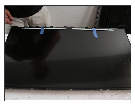
Flip up the buffer boards and tape them to the panel using suction cups.
