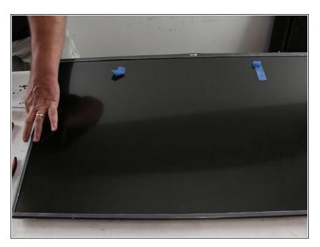
Reinstall the bezel and tighten it down using the screws that run around the perimeter of the TV.
