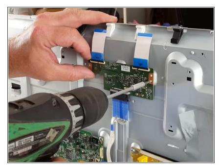
Some of the smaller tabs may be placed under the boards; to reach at least one of the smaller tabs, you will need to remove the t-con board.
