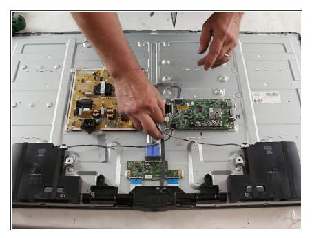
Reinstall the infrared sensor and tighten it to the chassis once more.
