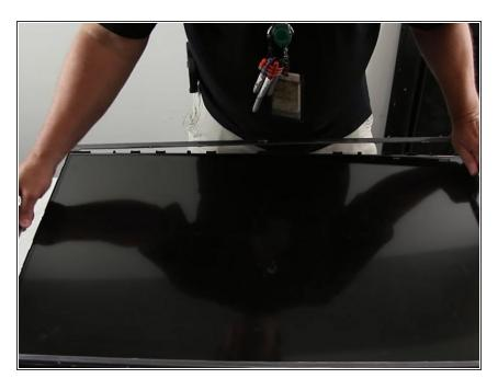
Remove the bezel by flipping the television over.
