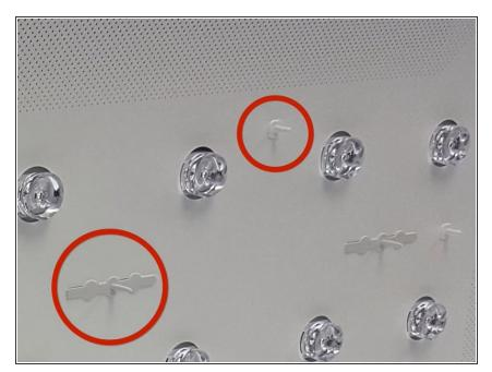
The reflector is held in place by two sets of tabs located on each side of it.
