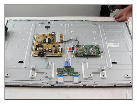
Remove the screws that hold the buffer board in place.
