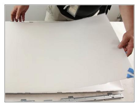
Tape the diffusion layers together at the corner to keep them aligned, then remove the layers of diffusion one by one, starting at the corner.
