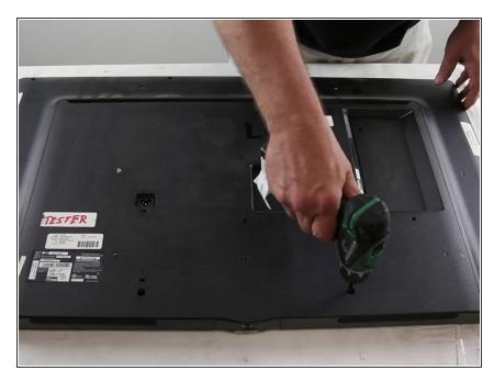
Remove the screws from the rear of the television, as well as the back cover.
