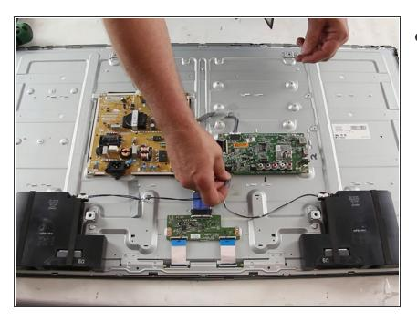
Reinstall the speakers and connect the wire to the mainboard.
