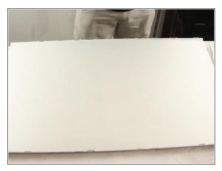
Remove the tape from the layers of diffusion and reinstall them.
