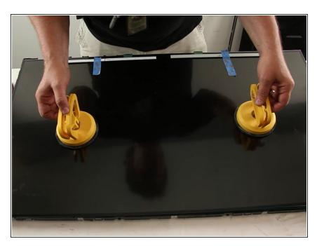
Adjust the panel's position and then remove the suction cups.
