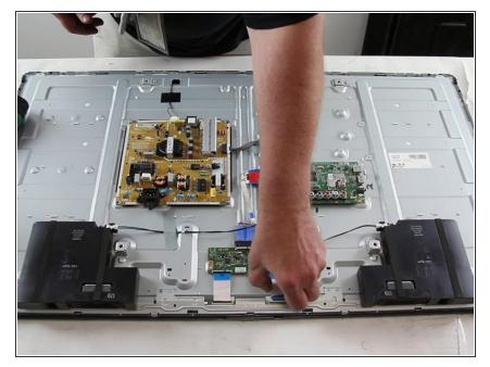
Remove the speakers from the mainboard by disconnecting them from it.
