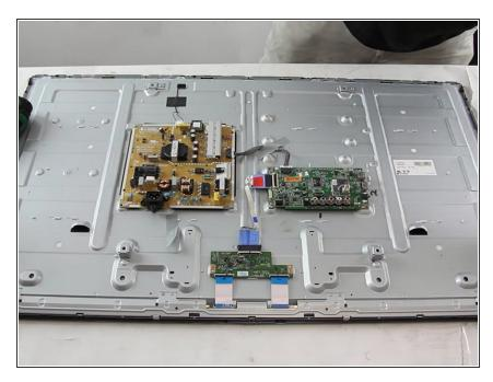
Remove the screws on the assembly that are around the television.
