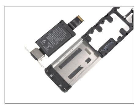
Remove the battery and charging port assembly. Compare your new replacement part to the original part—you may need to transfer remaining components or remove adhesive backings from the new part before installing.
