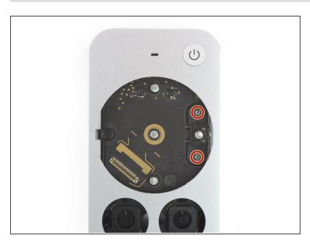
Use a T3 Torx screwdriver to remove the two 4.7 mm-long screws securing the Siri button on the right edge of the remote.
