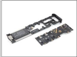
Lift the mainboard up and away from the battery to remove it.
