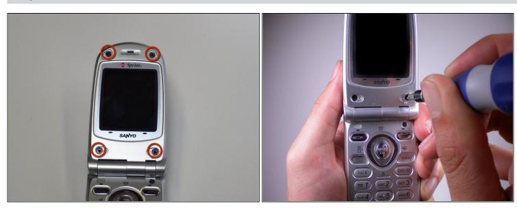
• Use the Tri-Wing Y1 screwdriver to unscrew the now uncovered four 0.5 mm screws.
