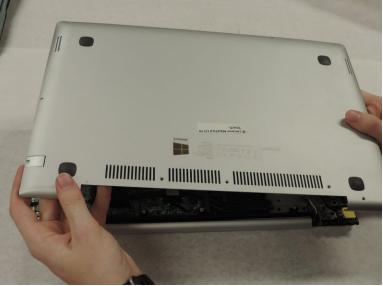
To remove the panel, use a plastic opening tool to prevent any damage.
