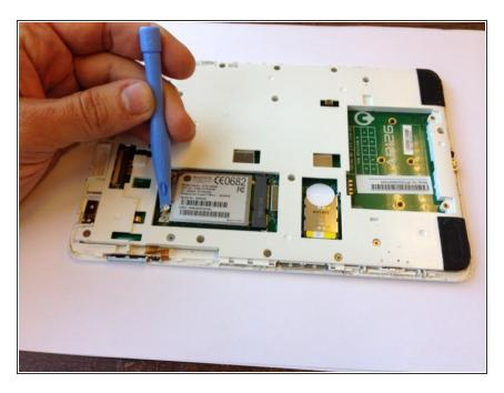
Use the plastic opening tool to wedge underneath the connection and gently pop off the wire cap.
