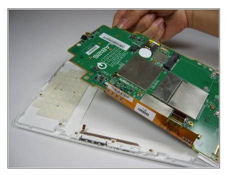
Grab the bottom corner of the motherboard and safely remove it from the Kindle.
