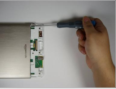
Use a Phillips #00 screwdriver to remove the two 4 mm screws from the metal casing.
