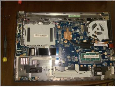
• Pull the hard drive out from the attachment to the motherboard.
