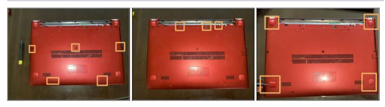
Remove the twelve screws from the rear panel.
