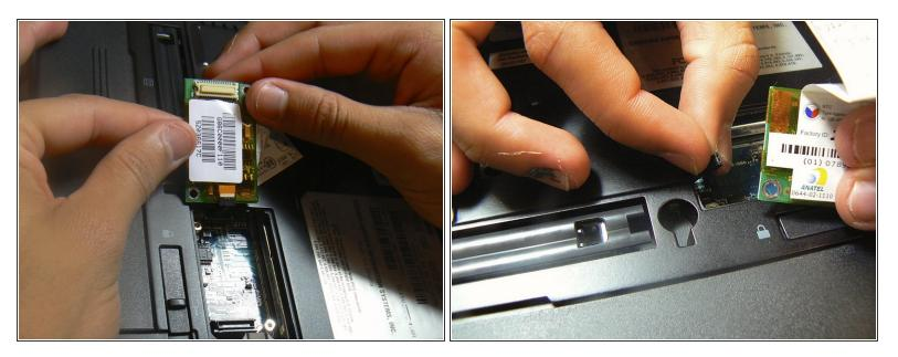
• Hold the edges of the wireless card and carefully disconnect the black 3 pin connector.
