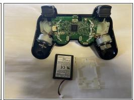
Carefully detach or disconnect the lithium polymer battery from the motherboard.
