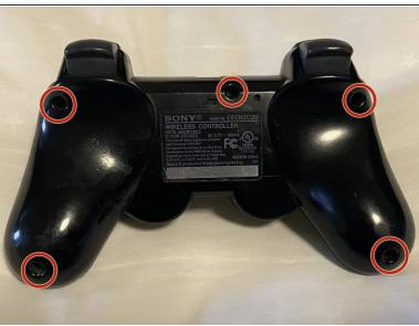
• Flip the controller over and locate the five 7.2mm Phillips #0 screws securing the rear cover to the front cover.
