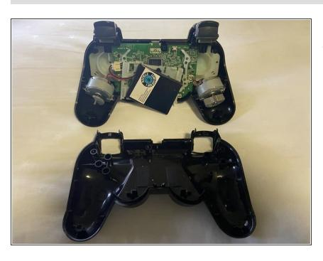
Lift the rear cover off of the controller to expose the interior.
