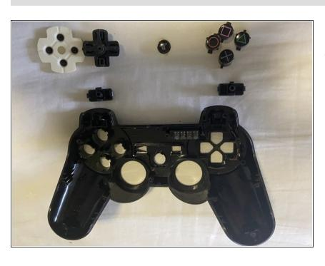
Set aside the colored buttons and lift the white rubber part holding the Dpad buttons in place to securely remove it. To reassemble your device, follow these instructions in reverse order.
