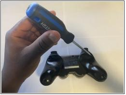
Using the Phillips #0 screwdriver, remove the five screws holding the rear/back cover in place.
