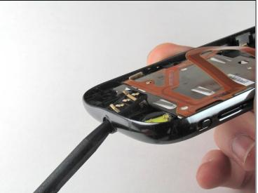
Gently insert the plastic spudger into the audio jack and pry upwards.
