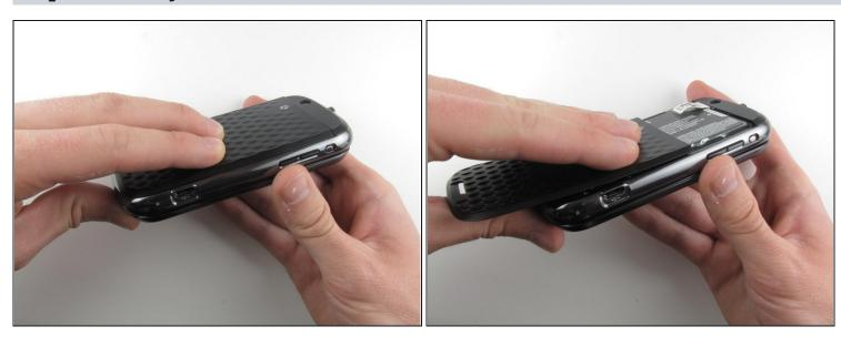
• Turning over your phone, place two fingers on the back cover and apply pressure away from the camera to slide the back cover off.
