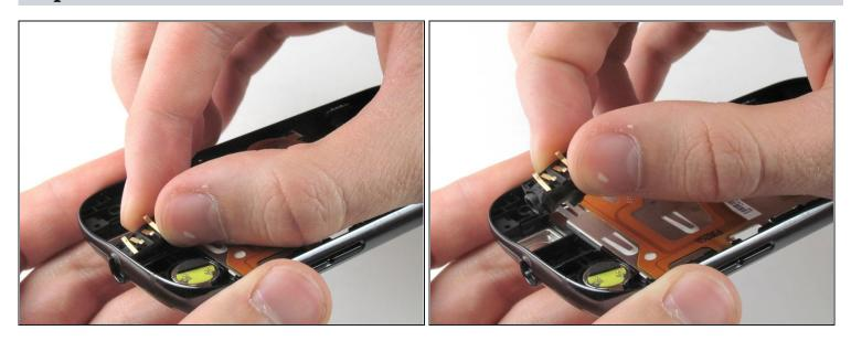
• Using your fingers, lift the audio jack out of its bracket.
