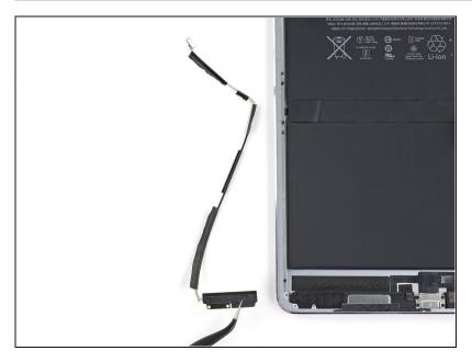
Remove the left antenna from the frame.
