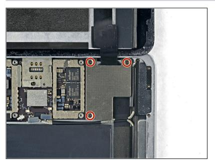
Use a Phillips screwdriver to remove the three 1.3 mm Phillips screws securing the display cable bracket.
