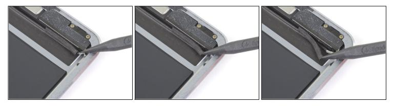
• Use the pointed end of a spudger to detach the foam spacer adhered to the fourth left antenna cable sticker.
