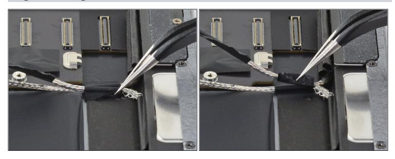
• Use a pair of tweezers to lift up the small sticker next to the lower right speaker securing the left antenna cable to the frame.
