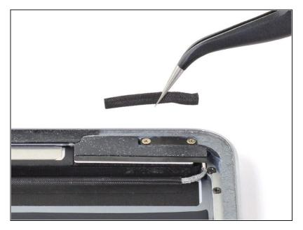
Remove the foam spacer from the fourth left antenna cable sticker.
