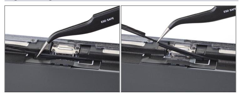
• Use a pair of tweezers to lift the left antenna and its third sticker away from the Lightning port area of the frame.
