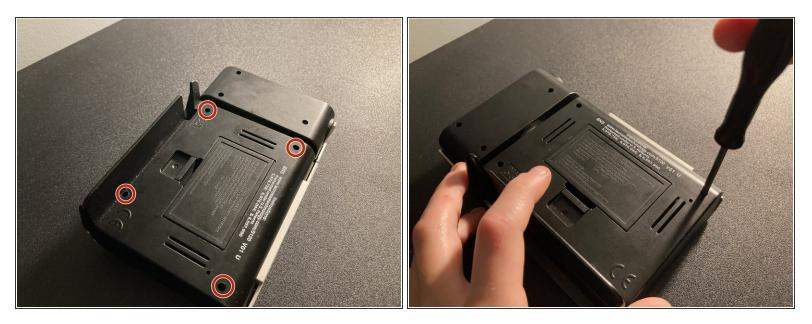
Before we get in, we need to remove the back screws. Use your THIN SHAFTED #1 Phillips Screwdriver.
