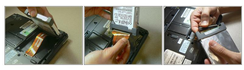
Carefully remove the hard drive from the IDE cable by pulling on the black connector.
