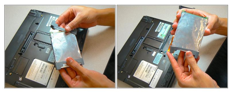
Remove the two gray rubber covers from both ends of the hard drive.
