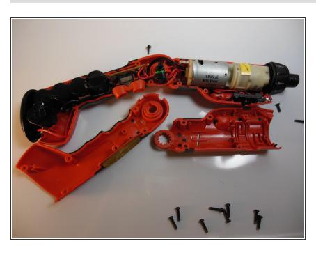
Lift one side of the drill casing off of the drill. Note that the drill casing consists of two pieces on either side of the drill.
