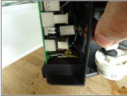
Pull the pump cable connector to disconnect it from the PCB.
