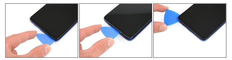
• Continue sliding the opening around the bottom right corner to the bottom left corner to detach the plastic clips.
