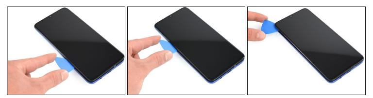
• Slide the opening pick along the left edge to detach the plastic clips.
