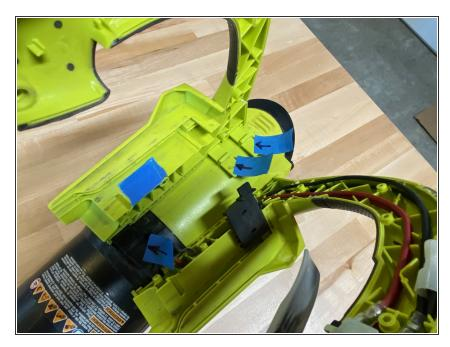
This view shows you the 3 alignment tabs. (see arrows on blue tape in picture) The handle slides onto these tabs. There will be no other clips or tabs.
