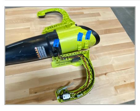
Wire routing is also simple. Wires are pushed into grooves in the handle. Remove wire harness and switch with a gentle tug.
