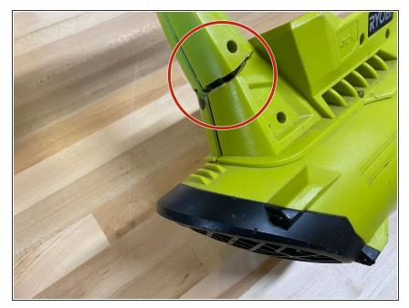
This style of handle can become cracked at the base. In this case it was broken almost completely through and very weak, but it can be replaced. This
