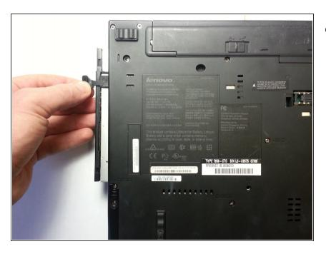
Once the tab pops out, pull it away from the computer to release the disc drive.
