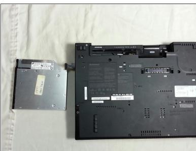
Pull the disc drive away from the laptop to fully remove it.
