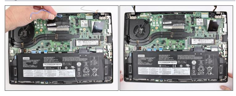
• Remove all antenna cables from their routing.
