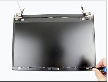
• Remove four 2.9 mm screws from the LCD panel using the Phillips #1 screwdriver.
