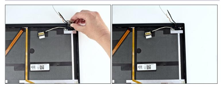
• Remove the hinge in the upper right corner.
