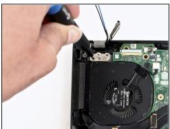
• Using the Phillips #1 screwdriver, remove three 5 mm screws from the left hinge and three 5 mm screws from the right hinge.
