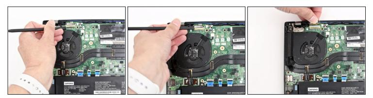
• Disconnect the camera cable from the motherboard using a spudger.
