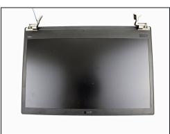
• Carefully rotate the hinges upward and remove the bottom of the machine from the LCD unit.
