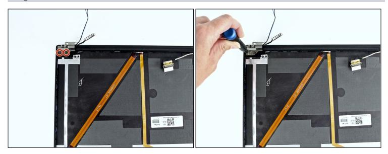
• Use a Phillips #1 screwdriver to remove two 2.8 mm screws from the hinge in the upper left corner.
