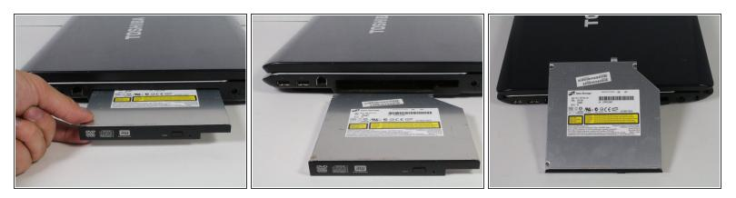
• Continue to pull the disk drive toward you until it is completely removed from the laptop's housing.
