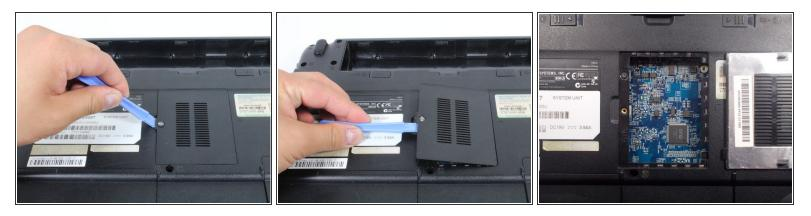
• Use a plastic opening tool to open the motherboard access cover.
