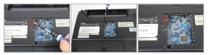
Remove one 1.5mm Phillips #1 screw located near the top left edge of the opening.
