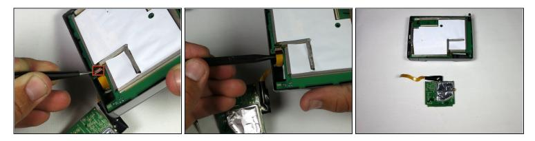
• Use the <u>tweezers</u> or the spudger to lift the tan latch off the ribbon cable (ZIF connector) and gently pull out the ZIF connector and cable from underneath the opened latch.
