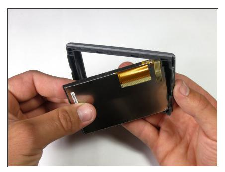
Finally, gently pull the screen out of the right side of the plastic shell.
