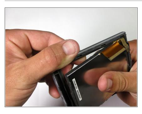
Once the top-left corner is out, carefully start detaching the bottom of the screen, starting from the bottom left.
