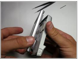
Detach the front display from the back panel of the device.
