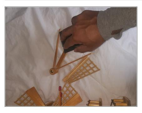
Use the rough sandpaper on parts that need to be connected to the primary unit as this will result in greater surface contact.
