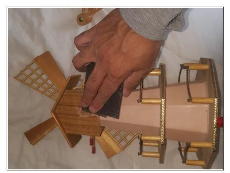
Use the 120 grit sandpaper to remove any rough edges on both the base unit and any parts which need to be connected to it.
