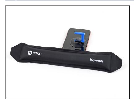
Apply a heated iOpener to the bottom edge of the display for one minute.
