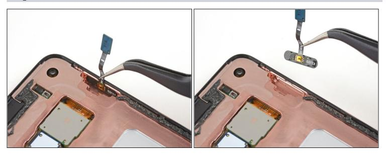
Remove the fingerprint sensor from its recess.
