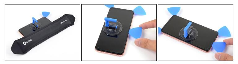
Repeat the heating and slicing procedure for the remaining display sides.
