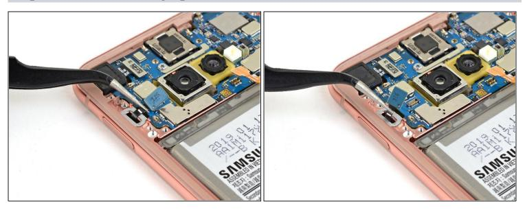
• Use a pair of tweezers to loosen the fingerprint sensor cable from the adhesive gasket.
