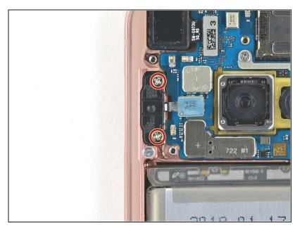
Use a Phillips driver to remove the two 4 mm screws securing the fingerprint sensor bracket.
