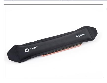
Apply a heated iOpener to the OLED panel for a minute to soften up the panel adhesive.
