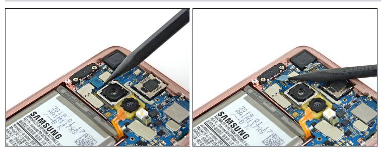
• Use the point of a spudger to pry up and disconnect the fingerprint sensor connector from its motherboard socket.
