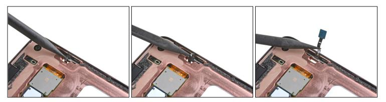
• Use the point of a spudger to gently pull the fingerprint sensor cable through its frame cutout.
