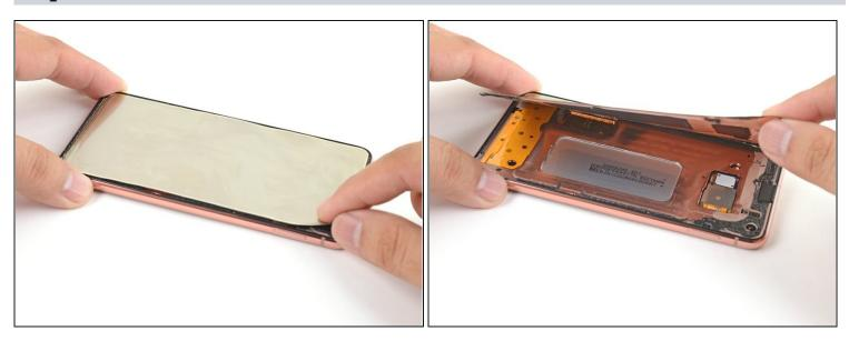
• Lift the display panel from the right edge and peel it away from the frame.
