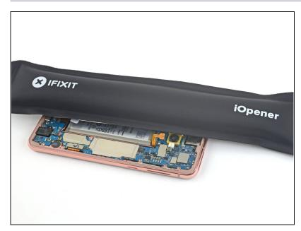
Apply a heated iOpener to the fingerprint sensor bracket for one minute to loosen the adhesive.
