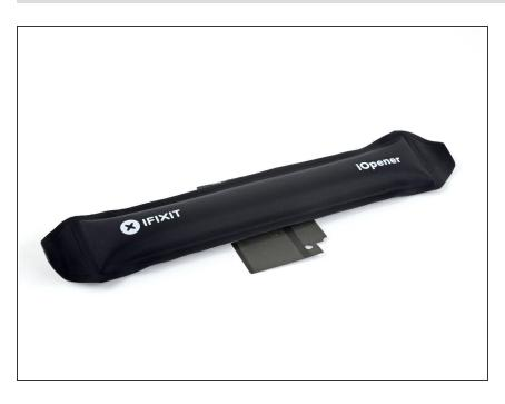
Apply a heated iOpener to the top half of the midframe for one minute.
