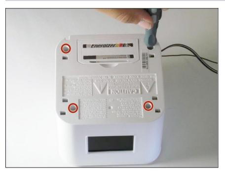
Remove the four screws from the base using a Phillips #1 screwdriver.
