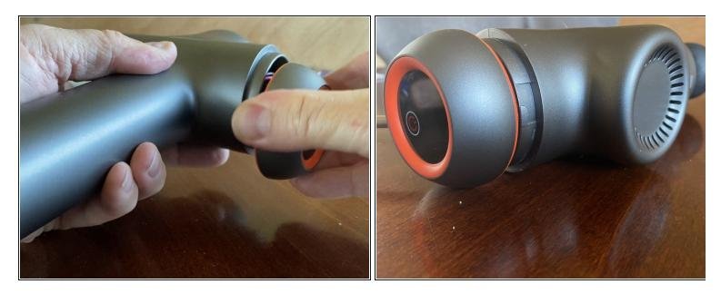
• Twist counter-clockwise very snug. It only moves about 1/4 of an inch - the second picture shows the slide lock slots.
