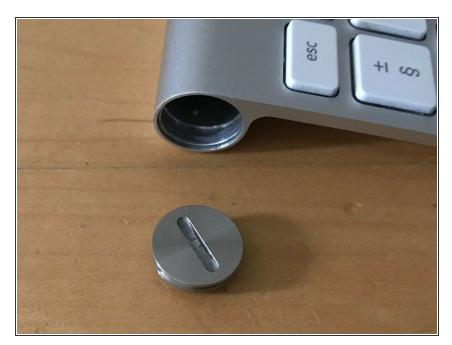
Using a flat object that fits into the slot, twist the cap clockwise to unscrew.
