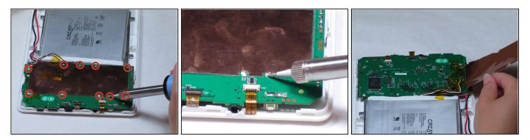
• Remove the copper plate covering the motherboard by desoldering the ten solder points.
