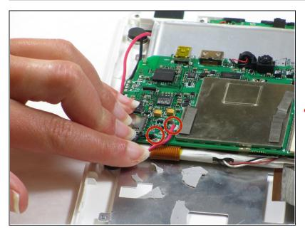
Remove the red and black wires with a soldering iron that are located underneath the motherboard.
