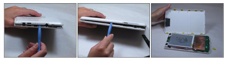
• Remove the back panel by using the plastic opening tool to carefully pry around the panel's edges.
