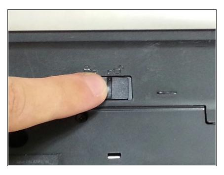
Use your finger to slide the release tab to the unlocked symbol.
