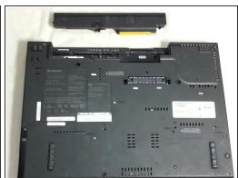
Hold the tab in the unlocked position and push the battery away from the computer to remove it.
