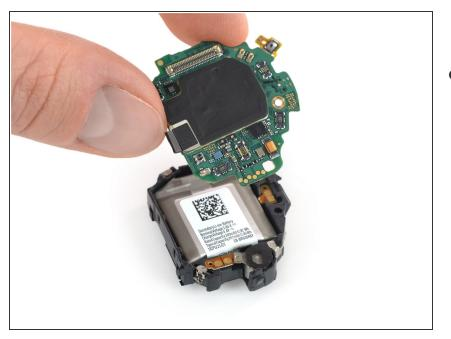
Slide the motherboard out from under the remaining plastic tabs to remove it.
