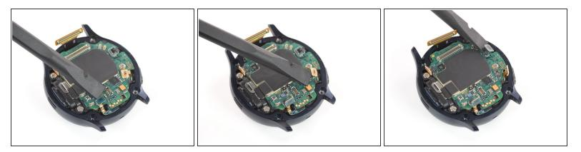
• Use a spudger to disconnect the barometric sensor, the buttons, and the microphone.
