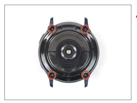
Use a Tri-point Y00 screwdriver to remove the four 4 mm-long screws on the back of the watch.
