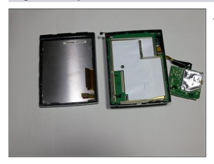
After following the instructions in the main dis-assembly guide, you should have the screen detached from the motherboard.
