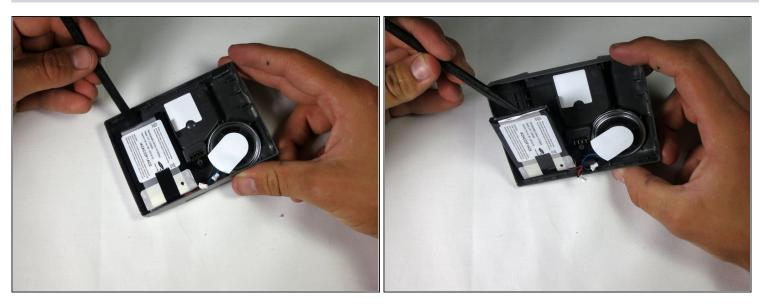
• Using the flat edge of the spudger from above, gently pry the battery away from the plastic.
