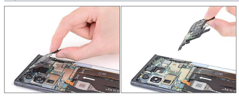
Lift and remove the earpiece speaker.
