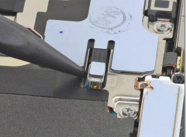
Use the pointed end of a spudger to pry up and disconnect the white press connector located in the bottom right of the motherboard shield.
