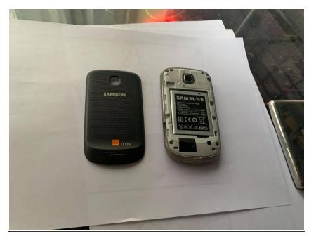
Very Easy, There is a Small hole below the Thick portion to pull the cover off
