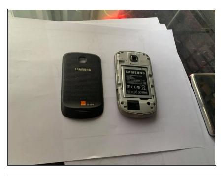
On The Lower Right there is a Small gap to pull the battery Out
