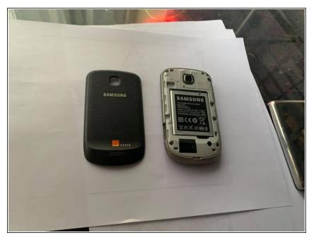
Under the thicker bit, there is a small spot to pull the Cover off
