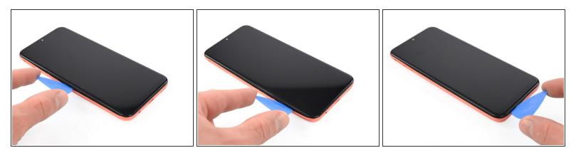
• Slide the opening pick around the bottom left corner to unclip the plastic clips.
