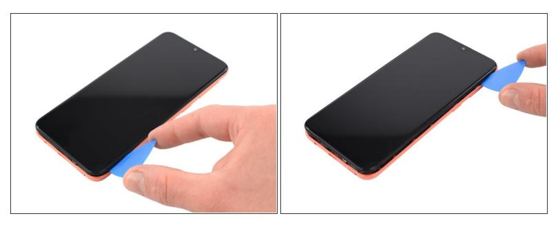
• Slide the opening pick along the right edge to the top right corner to unclip the plastic clips.
