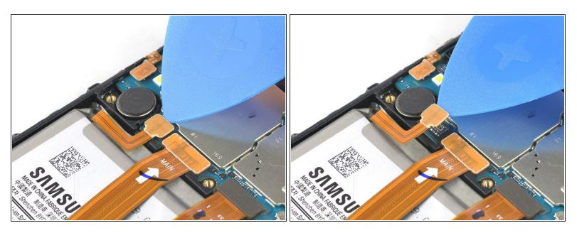
• Use an opening pick to disconnect the battery by prying the connector straight up from its socket.
