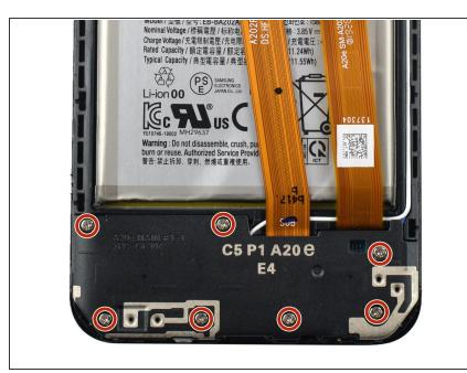
Use a Phillips screwdriver to remove the seven 3.5 mm-long screws securing the daughterboard cover.
