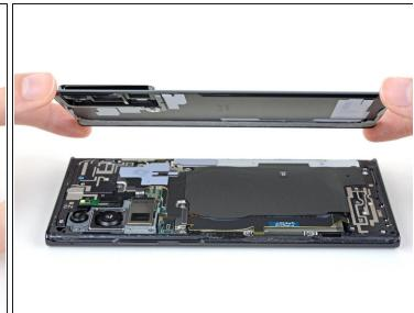
• Lift the rear cover straight up to remove it.
