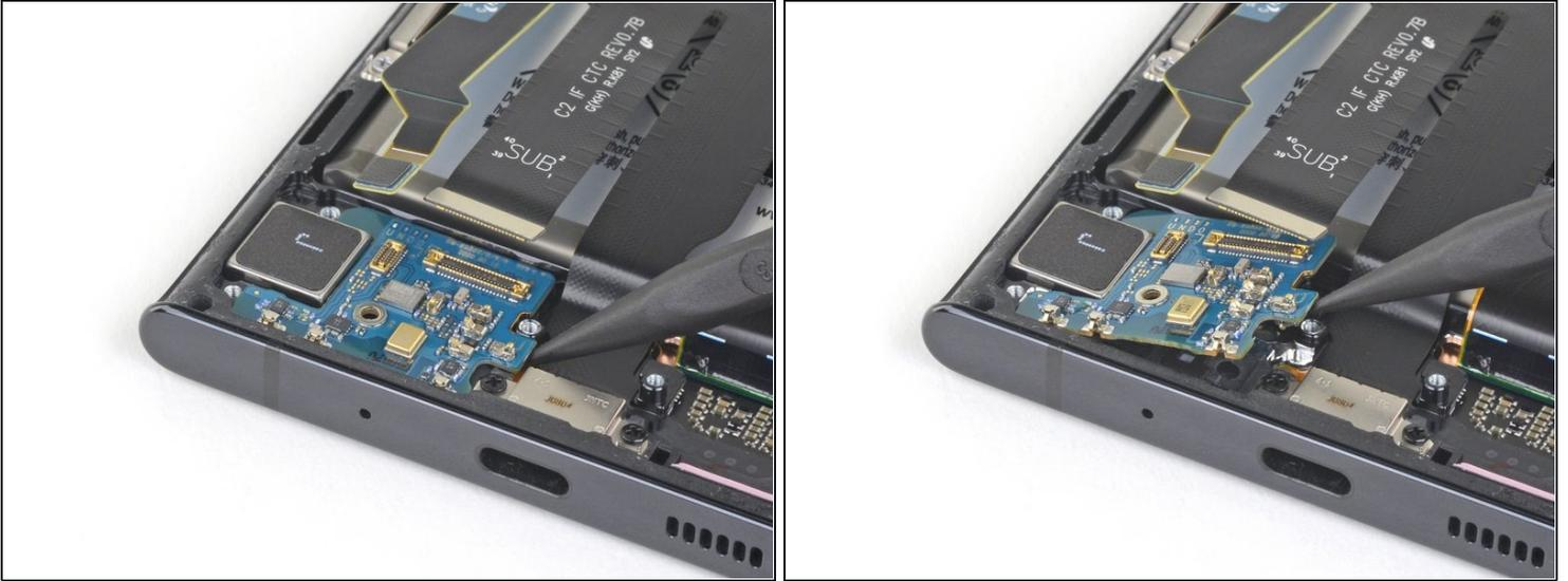
ⓘ The daughterboard is fitted to the frame by three spring connectors along its bottom edge.
