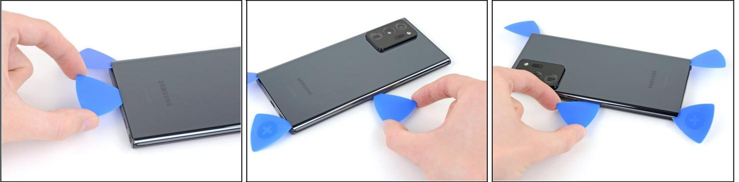
**⚠** While cutting through the adhesive, don't insert the opening pick more than 5 mm into the phone or you risk damaging the internal components.
