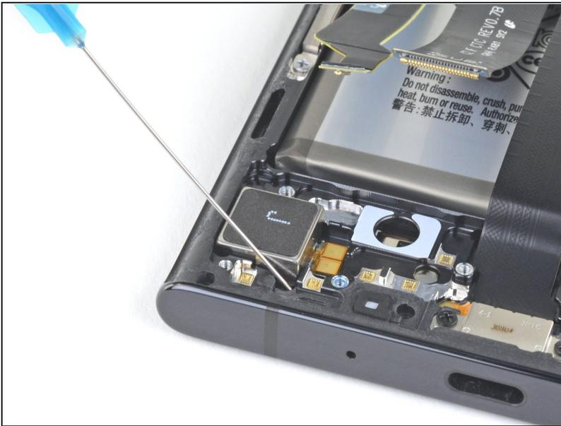
⚠ Do not scratch the copper pads attached to the vibration motor. Doing so may affect its functionality.
