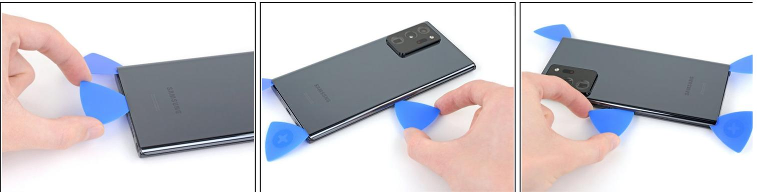
**⚠** While cutting through the adhesive, don't insert the opening pick more than 5 mm into the phone or you risk damaging the internal components.
