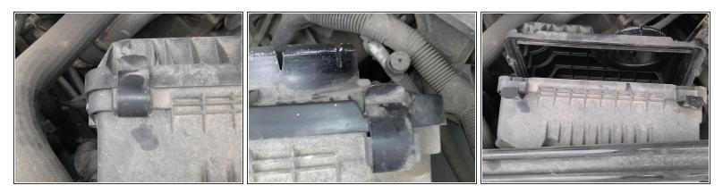
Undue the two tabs on the left and right sides of the filter box and lift the cover out.
