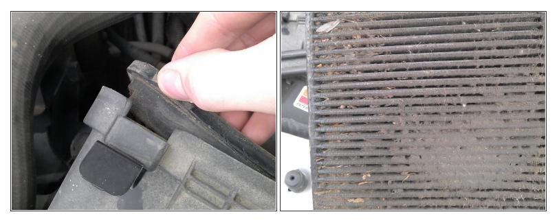
• Use the indent under the tab to pull the filter out.
