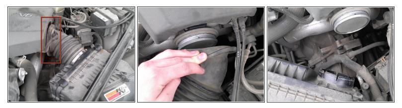
Simply tug on the rim of the tube and pull downward.
