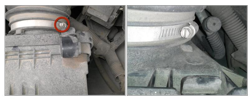
• Using the flat-head screwdriver, unscrew the brace until it is very loose. but not completely off!
